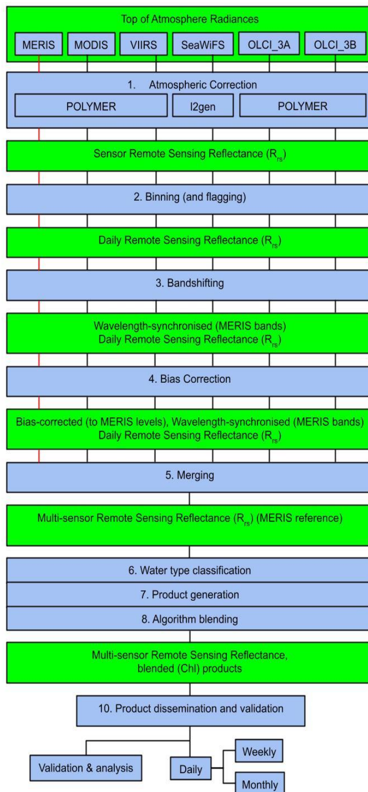
Figure 2: Data flow in the Ocean Colour ECV production process. Note that the atmospheric round robin is not part of the processing chain. It is performed once prior to the main data processing and the results are used to build the final processor configuration. As such it is not shown here as part of this process.
